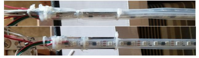
The strands are attached with a screw to the top plate. The bottom of the strands are held down with a Bungie (smallest available at Harbor Freight) to a 12 inch spike in the ground (lowes 12in spike). I use hundreds of zip ties which I get at Harbor freight. I also attached the two LED strips together along the length with a 3 inch zip tie but only barely snug. I used a drop of permatex silicone RTV to hold the zip
