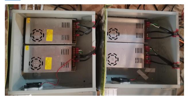
4x 42 Amp Power Supplies. I used tab Quick Disconnects that seemed to work well. I was prepared to switch to Anderson Powerpole connectors rated at 45 Amps. I added a ventilation port and some fans I found on Amazon. The wiring to the Tree strands is 10 Awg landscape wire with connectors.
